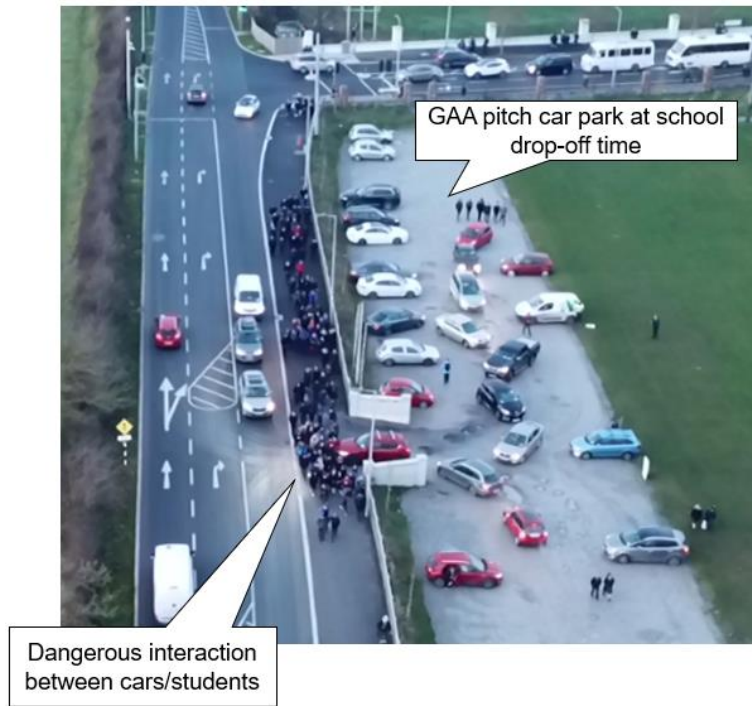
Figure 2.23 Drone Footage Indicating Dangerous Use of GAA Pitch Car Park as a Drop-Off Location for the MEC School Campus
